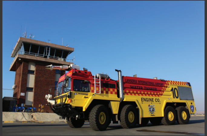
The refurbished Rosenbauer 8x8 Bush Panther Engine Company
